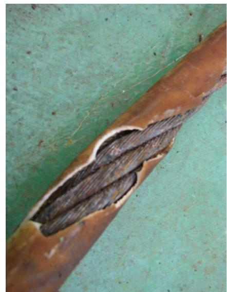
Figure 2. Corrosion beneath plastic sheathing.
