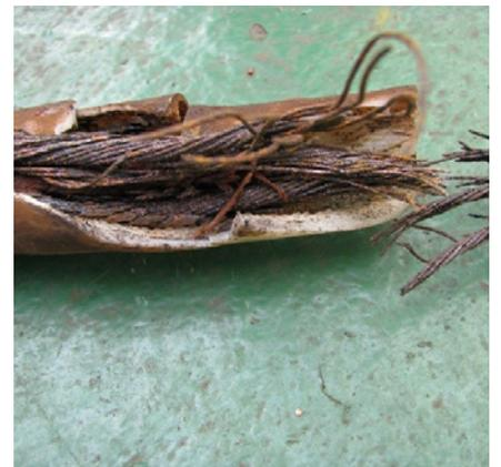
Figure 3. Lifting slings parted due to undetected corrosion.
